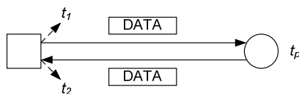
Fig. 2 Round Trip Time measurement between the blindfolded node and the reference node. Both time measurements are performed in the same node. This cancels out the need for synchronization. One cannot neglect the processing time ( t_p ) in the reference node.
