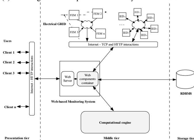
Figure 3: The proposed distributed architecture for power systems contingency analysis
