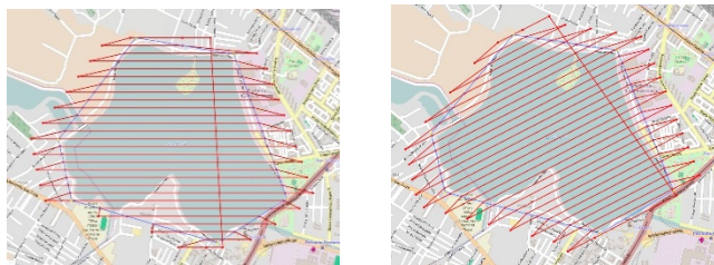
Figure 6. Line path generation over a real terrain feature
